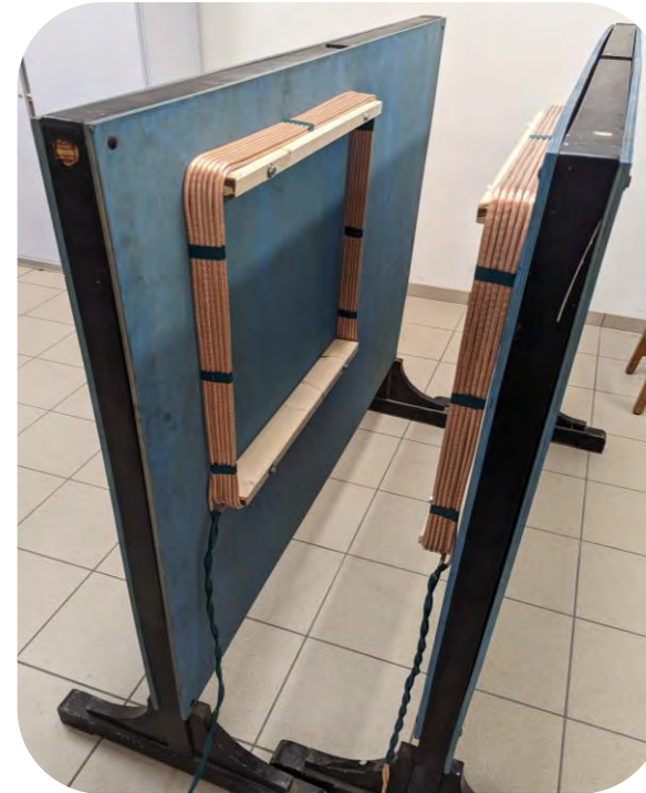
THE B FIELD GENERATION AND MONITORING SYSTEM
